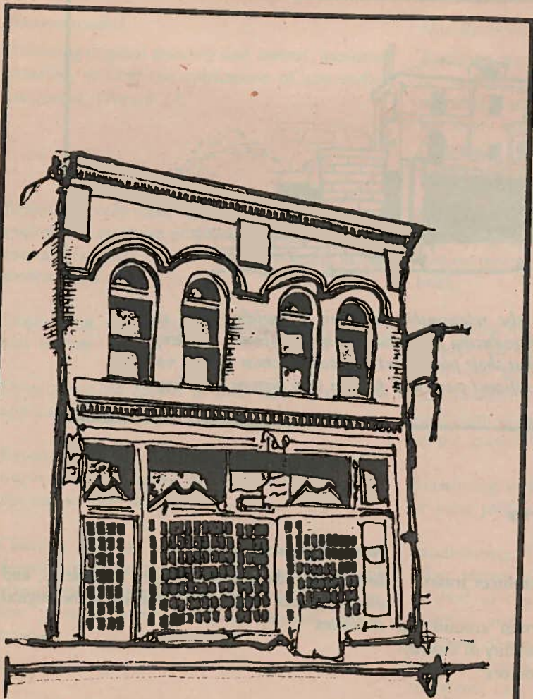
Avoid physical alterations which have no historical basis. The small-paned windows added to this 19th century western storefront are not accurate for this particular structure. (Figure 3).
